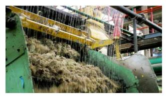
The crushed cane exiting the last mill is called bagasse. The juice from the mills is strained to remove large particles and then clarified.
