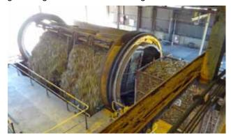
revolving knives, shredders, crushers, or a combination of these processes. For the grinding, or milling, of the crushed cane, multiple sets of three-roller mills are most commonly used although some mills consist of four, five, or six rollers in multiple sets. Conveyors transport the crushed cane from one mill to the next.
