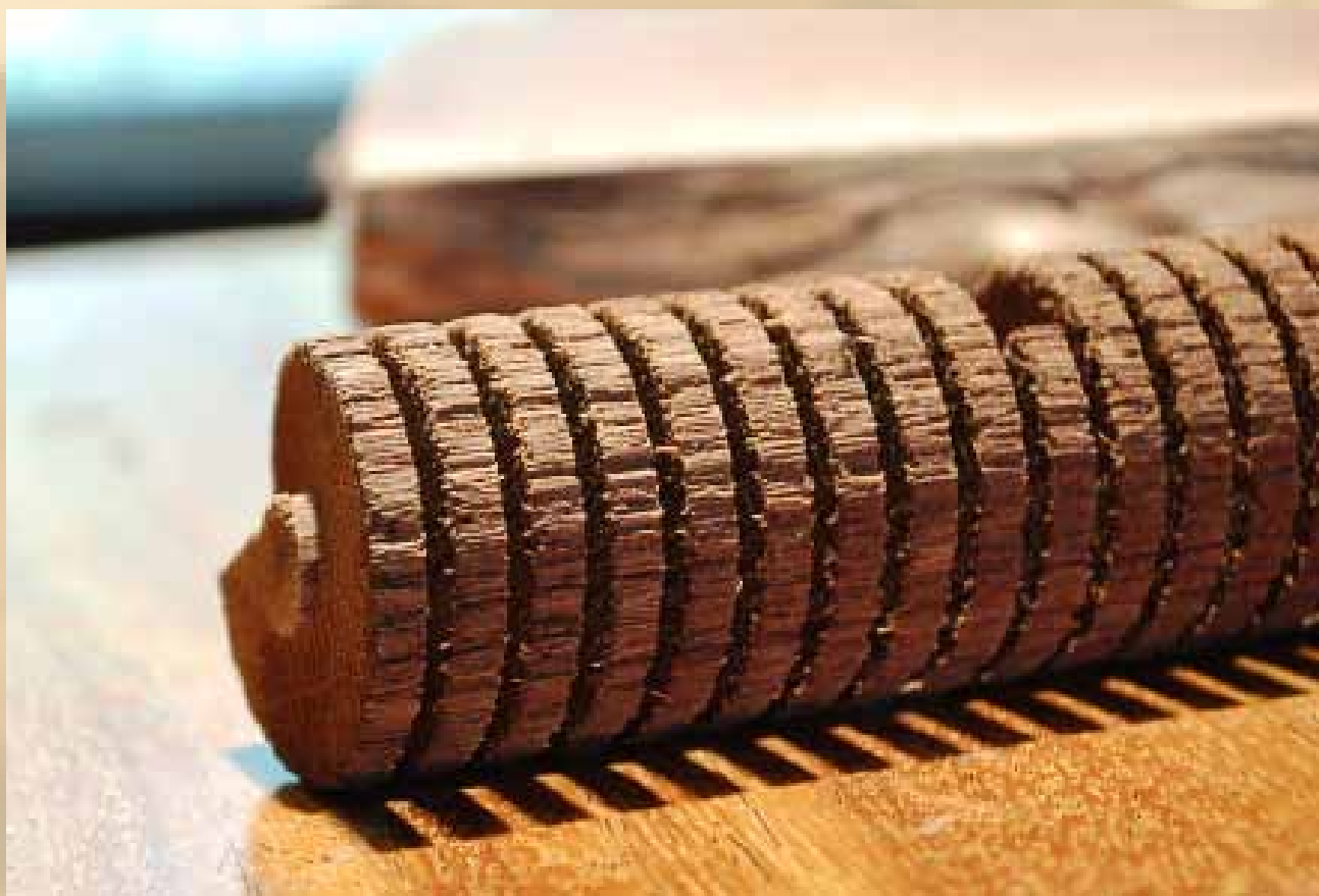
An oak spiral, designed to maximize the surface area oak exposed to the rum (Photo from LangdonWood)
