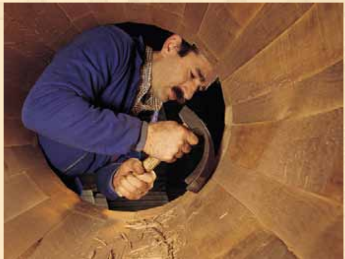
A master crafter carving the "croze" in a barrel, Viña Tondonia, Spain.
