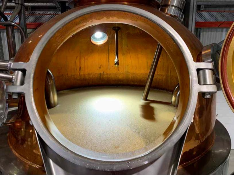
with the same equipment. We are distilling with a 528L steam jacketed Mueller pot still from Germany. It is an incredible machine, fast, precise with high reproducibility from one batch to the other. The manufacturer also promised that we would be able to distil 2000L in an 8-hour day shift. Their representative, Frank Deiter, agreed to travel 10,000 km to come and make sure we set it up correctly. With more than 400 distillations behind us, I could not be happier with our purchase.
