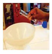
Glycerol is added using a measuring cylinder. As glycerol is very viscous and sticks to the wall of the measuring cylinder, it should be rinsed with some sterile distilled or cold boiled water and then emptied into the bottle/tank.
